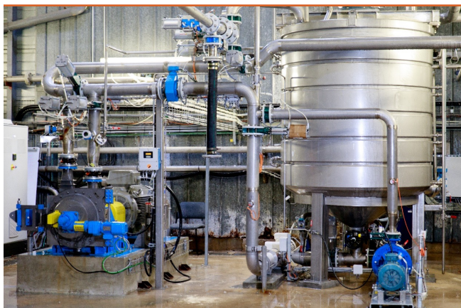
The Quad Hydradisc refiner at the Kadant Technology Center in Vitry-le-François
