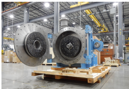
Quick-opening hinged housing with integrated plate crane provides safe and easy maintenance access
