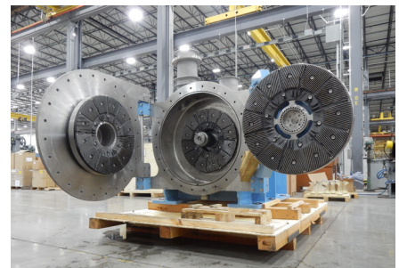
Quick-opening hinged housing with integrated plate crane provides safe and easy maintenance access
