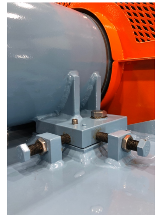
Easy field alignment of shaft and rotor
