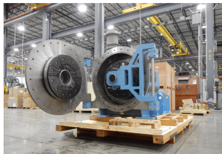
Quick-opening hinged housing with integrated plate crane provides safe and easy maintenance access
