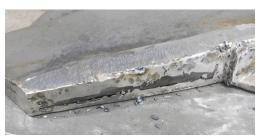
The damage is removed and the surface **prepared for reconstruction**.
