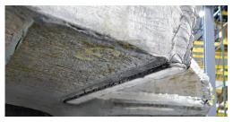
**KBC 51 Hard Weld** wear strips are added along the bottom of the rotor's leading edge and back towards the hub.
