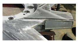
Additionally, all leading edges of the rotor vanes are wrapped with **KBC 51 Hard Weld.**
