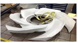
The rotors are then fully balanced and carefully **quality inspected** to ensure peak performance. They are then painted and packed for shipping.
