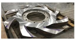
Rotors are rebuilt to an **optimized hydrodynamic geometry** based upon your application and the latest industry-leading Kadant performance innovations.
