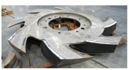
New face plates are fabricated from durable, wear-resistant **KBC Armor** and welded onto the rotor.
