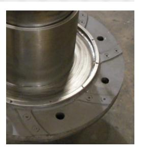
The underside of the hub clearly showing the wire barrier ring and bangor strips. A matching wear plate and packing box completes the upgrade.
