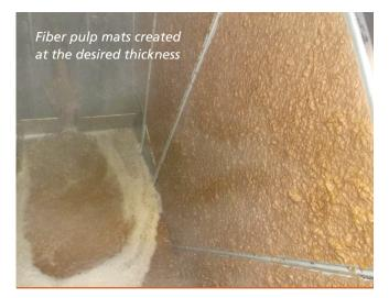
The main advantage over other dewatering equipment is that it retains most of the fibers.
