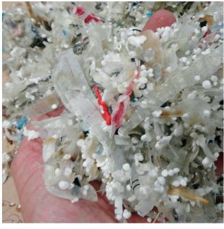
The slotted drum screen is excellent for the removal of styrofoam, one of the most abrasive contaminants found in recycling furnish.
