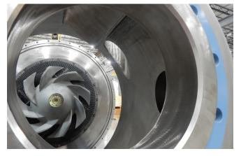
Designed smart and built tough for long-lived, dependable service – proprietary hardface-clad rotor and plates in a corrosion resistant, stainless steel body
