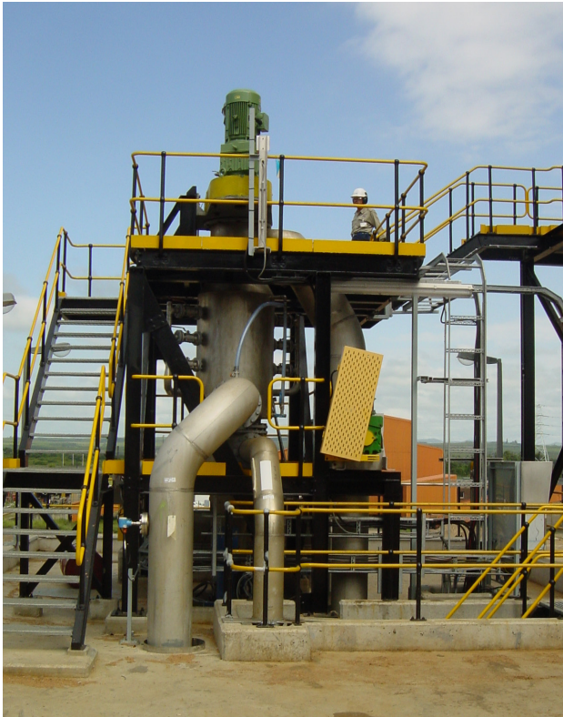
Raditrim-K secondary knotter screen installation
